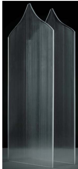
Figure 2: Sapphire sheet crystals growth via the edge defined film fed growth method at II-VI A&D, grown 12" wide and 30" in length.
