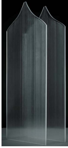
Figure 1: a) Typical sapphire sheet crystals produced from the EFG method at II-VI OS
